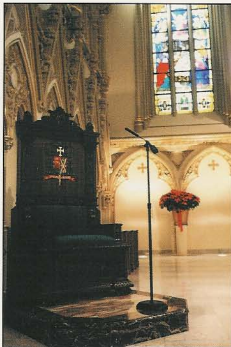
Figure 3 – A floor stand and mini-boom support an electret microphone at the Bishop's chair or cathedra.
